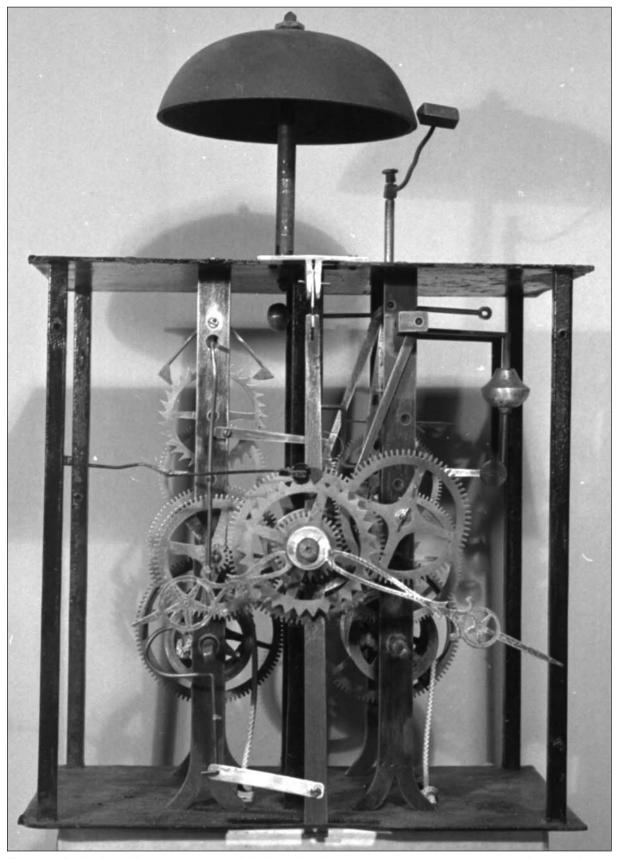
**Figure 2.** Behind the dial of a late model Morbier, showing the recoil escapement, and pendulum rod in front, with slotted brass suspension spring. This model also has a calendar mechanism.
